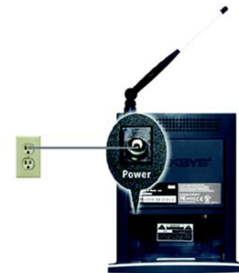
Figure 5-9: Connect the Power
